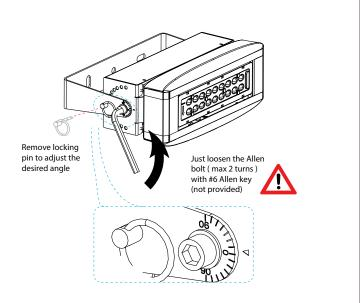
2. Mount the floodlight to the surface using one of the mounting options below:
