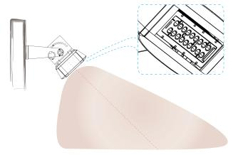
4. Tighten the bolts to fix the mounting bracket in position and secure with the bracket locking pin.
